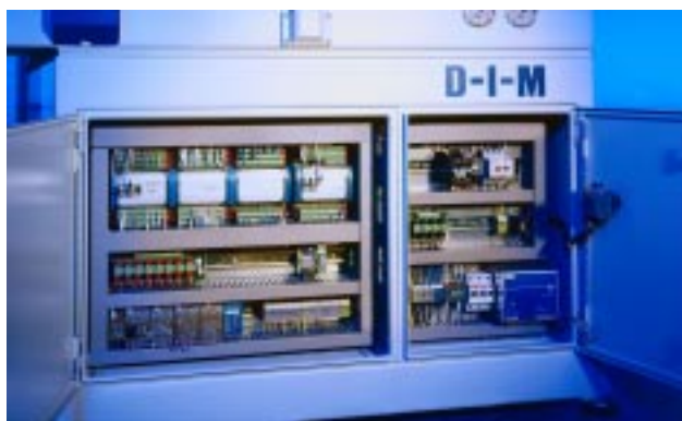
Fig. 1: Ettliger D-I-M control cabinet - “The complete automation system for of a multi-component injection molder is shown in this space-saving design, thanks to the compact, intelligent modules and the direct wiring to the sensors and actuators.”
